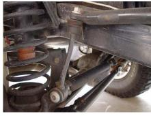
6. If you still have stock sway bar links on your Jeep, remove the bottom bolt and nut using an Torx T-55 Bit and 18mm wrench. If you have a set of aftermarket sway bar link disconnects, remove them using the tools specified by the manufacturer.
