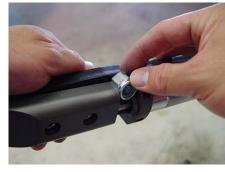
24. Hold the passenger side outer arm so that the air cylinder is facing you. Then, pull back the latch from the air cylinder and place one of the 1/2" nylock nuts that comes with the kit in between the two to hold it open.
