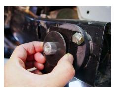
23. Back on the passenger side of your Jeep, place the large black plastic washer on the torsion rod.
