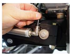
50. Take the longer 1/4" nylon air line and insert one end of it into the push-in fitting on your SwayLOC air cylinder closest to your front bumper.
