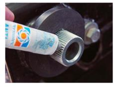
17. Go to the driver side of your Jeep, make sure the splines on the torsion tube are clear of any debris and then apply some Anti-Seize on it.
