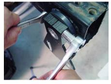
16. Insert a  $3/8 \times 2$ -1/2" bolt through the crosshole on the short passenger side arm and then attach a lock nut to the end of it. Using a 9/16" socket and wrench, fasten the nut to the bolt only to a snug fit at this time.
