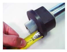
10. Take the torsion tube that came with kit and insert it through the urethane frame bushing so that the splines protrude 3/4" through it.
