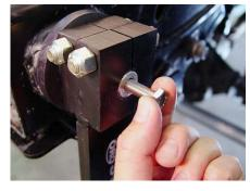
21. When the torsion rod reaches the driver side arm, thread in one of the 5/16-24 end cap bolts supplied with the kit and use the bolt to gently pull the torsion bar into the splines. Remove the bolt once the torsion bar is in the arm.
