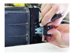
36. Using the air solenoid bracket as a template, locate and mark a place under the hood of your jeep where you will mount it. I decided to use the metal bracket on the driver side where a cruise control unit would normally be mounted. Since this location already has holes in it, I only needed to drill one new hole.
