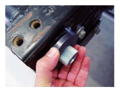
11. From the driver side of your Jeep, carefully insert the torsion tube and urethane frame bushing through the front cross member tube. Make sure the urethane bushing is sitting completely inside the frame tube. If needed, place a 1-1/4" socket over the torsion tube and use it to tap the urethane frame bushing into place with a rubber mallet.
