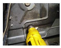
58. Make sure the carpeting inside your Jeep has been pulled out of the way along with anything else that might be on the floor of your Jeep. Then proceed to drill the air tank mounting holes using a 3/8" metal drilling bit.
