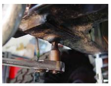
5. Again, using a Torx T-55 Bit, remove the 2 bolts (or 3/4" socket if you've already replaced these bolts) underneath your front bumper securing it to your Jeep's frame. Then, proceed to remove the front bumper off your Jeep and set if aside
