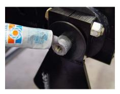
25. Once again, make sure the splines on the torsion tube are clear of any debris and then apply some Anti-Seize on it.
