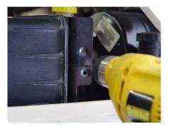
38. Drill your bracket mounting hole using a 5/32" metal drilling bit.
