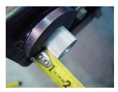
15. Double check to make sure the torsion tube is still only protruding 3/4" out of the driver side urethane frame bushing. If it's off, make whatever corrections you need by tapping the torsion ends with a rubber mallet
