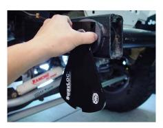
14. Carefully examine the splines on the short inner passenger side arm and clean out any debris you might find. Debris in the splines will make the installation of the arm onto the torsion tube quite difficult. Then, with the decals facing you and the notch on the end of the arm pointing towards the ground, slide it onto the splines of the torsion tube. If needed, use a rubber mallet to gently tap it into place.
