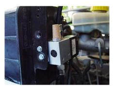
62. Cut the 1/4" nylon air line and insert it into the SwayLOC air solenoid push-in fitting labled "IN". Also, be sure to install the muffler on to the exhaust port of the air solenoid.
