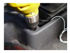
45. Route the white wire you fed into the cab of your Jeep under the center console. Then drill a 3/4" hole into your console or wherever you want to install the SwayLOC switch. I would recommend using a unibit for this job as it will drill a very clean and accurate hole.
