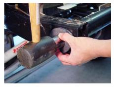
12. Apply some Viper Lube on the other urethane frame bushing that comes with your kit and install it on the passenger side of your Jeep's. Again, if needed, place a 1-1/4" socket over the torsion tube and use it to tap the urethane frame bushing into place with a rubber mallet.
