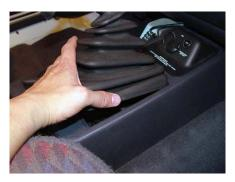
44. Climb back into your Jeep and remove the rubber transmission shifter boot by carefully pushing in the sides and lifting up. With a little effort, it should pop out without the assistance of tools.
