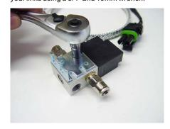
35. Back at your workbench, open the package containing the SwayLOC air solenoid and install the mounting bracket onto it using the self-tapping bolts provided. You will need a 1/4" socket for this job.
