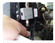
54. Cut the 1/4" nylon air line and insert it into the push-in fitting labeled "OUT" on your SwayLOC air solenoid. This fitting should be located next to the wiring harness. If you have on-board air, insert the remaining air line into the push-in fitting labeled "IN" and then route it to an air manifold connected to your compressor.
