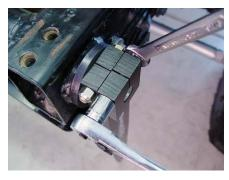
22. Insert a 3/8 x 2-1/2" bolt through the remaining cross-hole on the driver side arm and then attach a lock nut to the end of it. Using a 9/16" socket and wrench, fasten the nut to the bolt only to a snug fit at this time.
