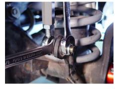
34. Again, using a 5/8" and 3/4" wrench, attach the SwayLOC links to the inside of the sway bar mounts on your Jeep's axle and then secure them in place using the nylock nuts provided with the kit.
