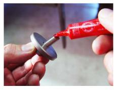
29. Once the end caps have been fitted properly, remove them, add a single drop of red Lock-Tite to each bolt and then re-install them onto their appropriate sides on your torsion bars. Then, go through and tighten each of the 3/8" nuts and bolts to 40 ft. lbs. of torque. Also, you can re-install your front bumper and winch at this time.
