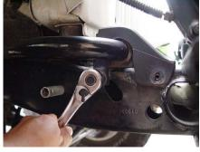
3. If you do not have a winch, you will need to remove the front plastic cover with the Jeep logo on it. The cover is secured by 2 bolts on either side of your Jeep and you will need a 10mm socket to remove them.
