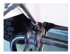
7. Using a 15mm socket and ratchet extension, remove the 4 bolts securing your Jeep's antisway bar to your frame. With the bolts removed, you should be able to just lift the antisway bar up and off your Jeep. With everything off, I would use this opportunity to clean up any mud build up or other debris that has built up in this area
