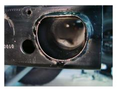
8. Carefully clean and inspect your front cross member tube on both sides of your Jeep making sure that the surface inside is smooth. On some Jeeps, you will find welding slag inside the tube and these will need to be ground off with a Dremel prior to installing your new SwayLOC System.
