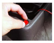
47. Snap the red activator switch into place and then feed the power and ground wires through the center console towards the firewall. Reinstall the transmission shifter boot back onto the center console.
