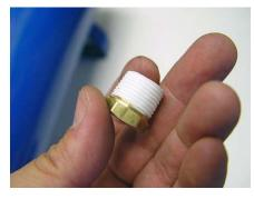
55. If you do not have on-board air and purchased the optional air tank with your SwayLOC System, you will need to begin assembling it now. Go back to your workbench, apply some teflon tape to the brass reducers and install them onto the tank using an 11/16" wrench.
