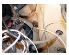
41. The air solenoid should have come with a separate two prong connector that has a white and black wire with a ring on the end of it. Feed the white wire through the hole you just drilled in the rubber plug on your firewall. Then, inject the hole with a little silicon sealer to close it off.
