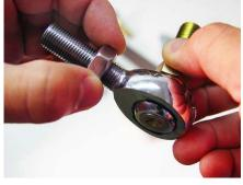
30. Back at your work bench, begin assembling your SwayLOC links by installing a jam nut on to each of the rod-ends.
