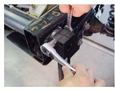
19. Insert a  $3/8 \times 2-1/2$ " bolt through the crosshole closest to the frame on the driver side arm and then attach a lock nut to the end of it. Using a 9/16" socket and wrench, fasten the nut to the bolt only to a snug fit at this time.
