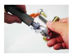
31. Install the rod-ends onto the hex aluminum housings provided with the kit.
