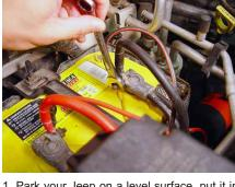
1. Park your Jeep on a level surface, put it in gear and engage the emergency brake. If you have a winch on your Jeep, open your hood and disconnect the 2 leads attached to your battery. The entire winch and mounting plate will need to be removed to complete the installation of your new Off Road Only SwayLOC Anti-Sway Bar System.
