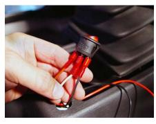
46. Take the red activator switch and feed the red power and black ground wire through the hole you just drilled. Feed the white wire coming from the air solenoid up through the hole and plug it into the center prong on the switch.
