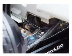
53. Route both air lines across your Jeep's front grill using zip ties to hold it in place. The shorter air line should stop here but continue to route the longer hose along your Jeep's frame rail and up into the engine compartment where your SwayLOC air solenoid is located.
