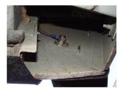
42. Attach the black wire with the ring connector to your Jeep's frame or body. I attached mine to a rocker guard bolt on the body of my Jeep.
