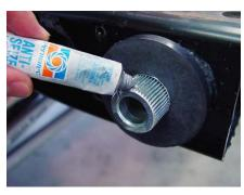
13. Back on the passenger side of your Jeep, make sure the splines on the torsion tube are clear of any debris and then apply some Anti-Seize to it.
