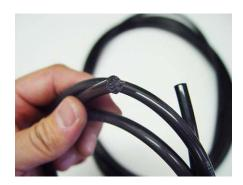
51. Take the shorter 1/4" nylon air line that has one of the ends melted closed and insert the open end into the push-in fitting on your SwayLOC air cylinder closest to the latch. Keep the length of air line whole and Leave the melted end intact. This air line will allow the air cylinder to move but keep dirt, mud, moisture from getting into it.
