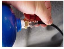
61. Insert the remaining 1/4" nylon air line into the push-in fitting pointing towards the front of your Jeep and route it along the driver side frame rail toward the engine where the SwayLOC air solenoid is located.
