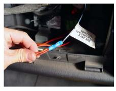
48. Remove your glove box to gain access to the fuse box. The SwayLOC kit should come with a fuse tap so that you can piggy back the fused side of a 10 amp fuse but if your Jeep comes equipped with an auxiliary switched power lead, you can attach your power wire directly to it. The SwayLOC air solenoid draws less than 300ma.
