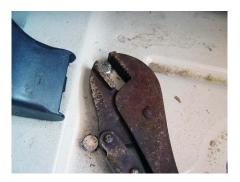
59. Inside the cab of your Jeep, take your 5/16-18x1 stainless steel bolts, slip a washer on them and insert them into the holes you just drilled. Place a pair of vice-grips and clamp it onto one of the bolt heads.
