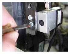
39. Install your air solenoid onto the bracket using the bolts and spoked nuts provided with the kit. You will need a small flat head screwdriver to secure the bolts in place.
