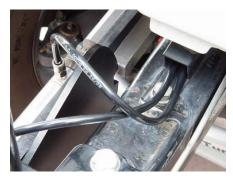
52. Make sure to leave a service loop on both air lines to allow for adequate movement and then secure them in place with a zip tie.
