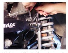
33. Using a 5/8" and 3/4" wrench, attach the assembled links on to the outside of the SwayLOC arms and secure them in place using the nylock nuts provided with the kit. If your jeep has wheels with more than 4" of backspacing, you may need to install the passenger side link on the inside of the SwayLOC arm.
