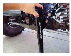
18. Carefully examine the splines on the driver side arm and clean out any debris you might find. Then, with the decals facing you and the end of the arm pointing down to the ground, slide it onto the splines of the torsion tube. If needed, use a rubber mallet to gently tap it into place.
