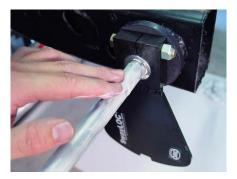
20. Apply a generous amount of Viper Lube to the torsion bar and then slide it into the torsion tube from the passenger side of your Jeep. Rotate the bar and continue to apply more Viper Lube to the torsion bar as its being fed in to insure good coverage.
