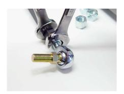
32. Adjust the overall length of each link so that the arms will not limit the front suspensions droop or make contact with the fender area when compressed. Measure the gap between your bump stops and lower spring perches to determine the approximate up travel your SwayLOC arms will make. Be sure to account for the compression of the rubber stop. Fasten your links using a 3/4" and 19mm wrench.
