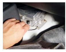
49. Lift up the carpeting on the passenger side of your Jeep and route the activator switch wires underneath it. Then, attach the ground wire to a bolt on your tub that will provide a good ground.
