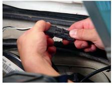
43. Plug the air solenoid wiring harness into the two prong connector and then zip-tie the wires up against the firewall.
