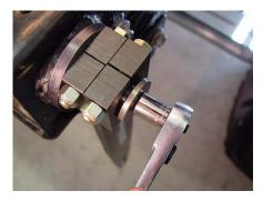
27. Place the larger of the two gray anodized aluminum washers onto one of the 5/16-24 end cap bolts and then secure it to the end of the torsion bar on the driver side arm using a 1/2" socket
