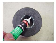
9. Take one of the urethane frame bushings that comes with your kit and apply some Viper Lube onto the inside surface of it. A small tube of Viper Lube should have been included with your kit.
