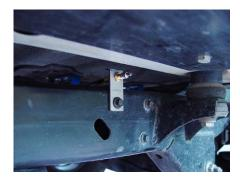
63. Using a piece of 1"x1/8" stainless steel bar stock, I made a bracket that I could attach the schrader valve to and mount it to my Jeep's driver side frame rail using an existing bolt (previously used for a side step).
