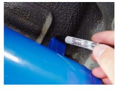
57. Climb under your Jeep from the driver side and hold your air tank up to the tub, parallel to the length of the Jeep and just behind where the driver seat would be. Use the air tank as a template and mark off where you will be installing it and where you will need to drill the mounting holes.
