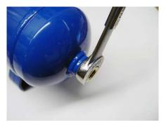
56. Install the 1/4" NPTs to the 1/4" tube fitting using a 9/16" wrench. The optional tank should only have one of these and your SwayLOC kit should have come with the other one you need.
