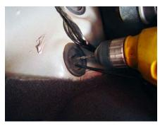
40. If you look under the dash on the driver side of your Jeep, you should see a large rubber plug on the firewall above the gas pedal and towards the center console. Drill a small 1/4" hole through this plug. As you can see in this photo, I already have a cable for my hand throttle going through it.
