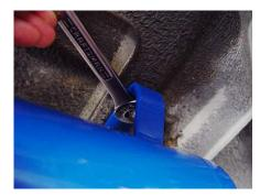
60. Back underneath your Jeep, secure the bolt that is clamped with a nylock nut. You will need a 1/2" wrench for this job.
