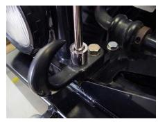
4. Using a Torx T-55 Bit (or 3/4" socket if you've already replaced these bolts), remove the 4 bolts securing the top of your front bumper to your Jeep's frame, along with any two hooks you might have. If you have a winch, you will need to remove it and its mounting plate completely from your Jeep.
