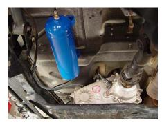
64. Take the remaining 1/4" nylon air line, insert it into the air tank's rear push-in fitting and then route it to your schrader valve's push-in fitting.
