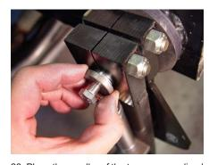
28. Place the smaller of the two gray anodized aluminum washers onto the other 5/16-24 end cap bolt followed by a 5/16 flat washer and then secure it to the end of the torsion bar on the passenger side arm using a 1/2" socket. Make sure that the bolt does not bottom out prematurely. If it does, add another 5/16 washer to make up the difference.
